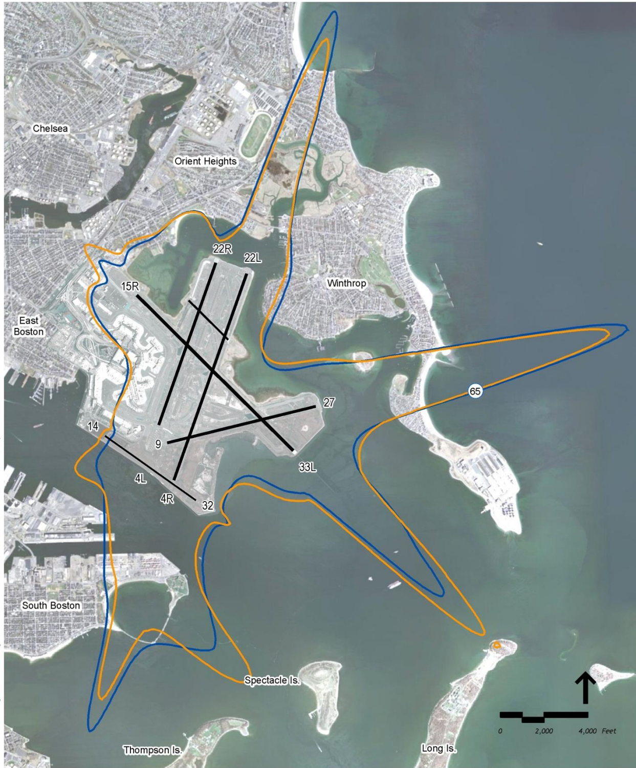
Comparison of the DNL 65 dB Contours for 2012 Operations Using INM 7.0c and 2013 Operations Using INM 7.0d
