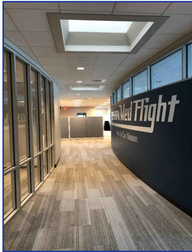
Figure 11-6 Boston Medflight Facility Utilizing Large Skylights for Day-lighting
