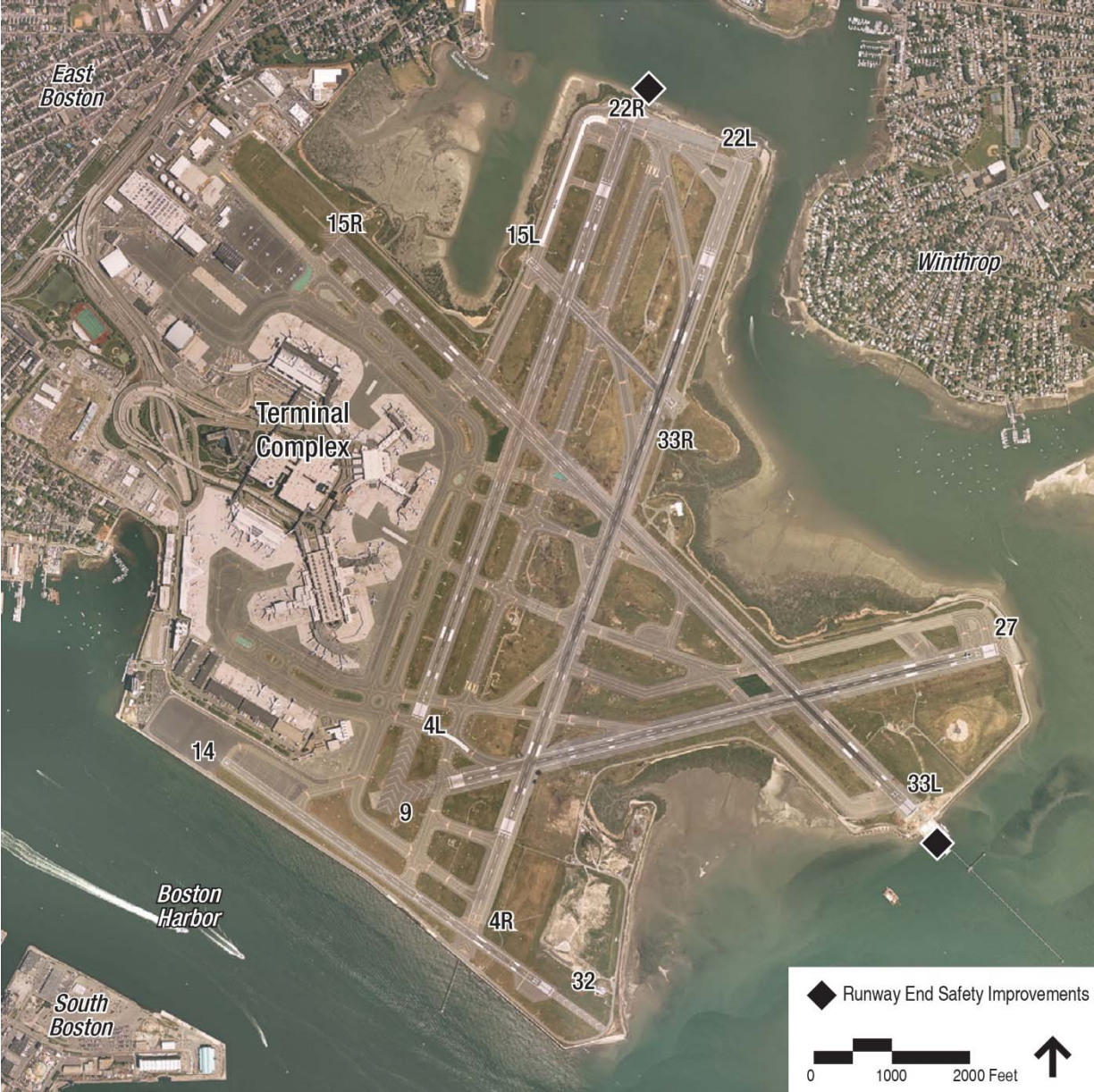
Figure 9-5 Runway End Safety Improvements
