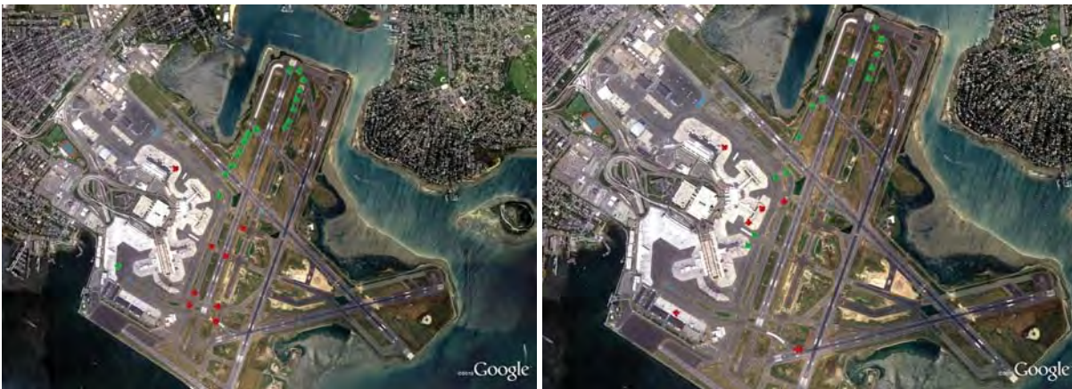
Figure 10: Snapshots of the airport surface, (left) before metering, and (right) during metering of pushbacks. Departing aircraft are shown in green, and arrivals in red. We note that the line of 15 departures between the ramp area and the departure runway prior to commencement of pushback rate control reduces to 8 departures during metering. The white area on the taxiway near the top of the images indicates the closed portion of taxiway “November”.
